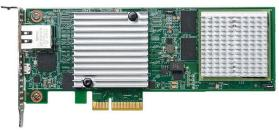
M820L is a media accelerator card that can be attached to server system to accelerate codec processes without changing existing users' server configuration.
