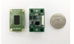
Photo: Radar Flight Control Module (RFCM) View larger image
