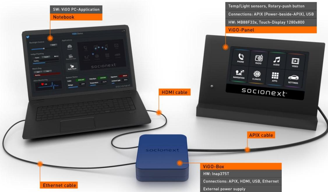
Fig 1: ViGO | Remote Display Demonstrator Showing Functional Safety
