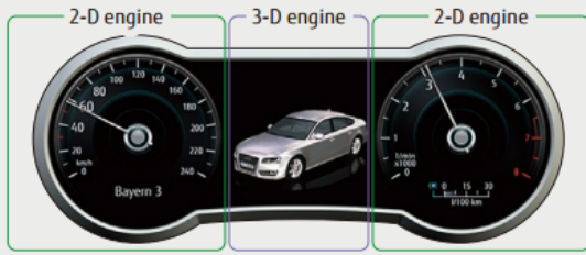
Figure 8 Rendering the needles of cluster display and the image of the vehicle
