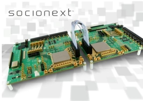
Photo 1: Socionext’s Rotta (ADC) / Oola (DAC) Development Kit designed and developed within the framework of Celtic-Plus SASER project. ([view larger image](#))
